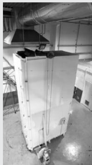
Example of CPD test chamber acc.to prEN50399
