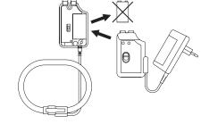
Bring unlimited autonomy to your Amp**FLEX**<sup>TM</sup>: replace the battery with the mains adapted plug
